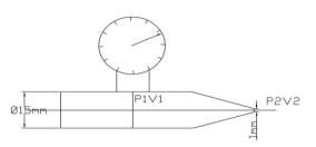
Fig. 1: Nozzle Arrangement – line diagram for Test Rig By applying Bernoulli's equation, at point1 and at point2
