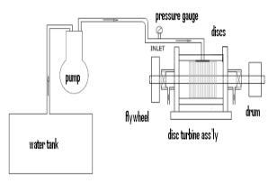
Fig. 4: Experimental Set up.
