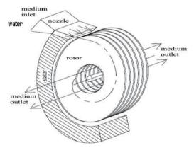
Fig. 3: Cross Section of Test Rig
