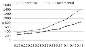
Flow Lit/s Fig. 5b: A plot of Flow v/s Speed for 6 smooth discs and 0.55mmn spacing
