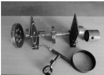
Fig. 2: Parts of Multiple disc Turbine.
